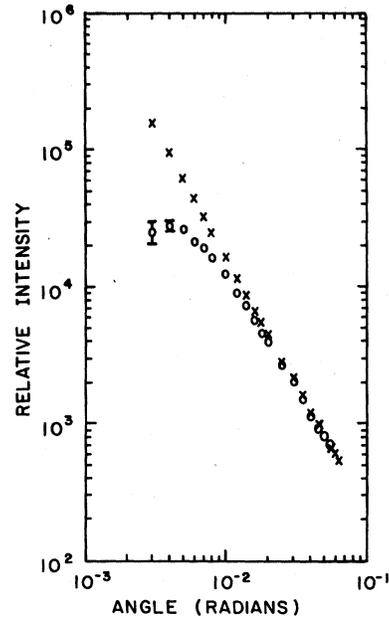
FIG. 1. Scattering curves, corrected for collimation effects and background scattering, for the one-phase region at temperatures  $0.01^\circ\text{C}$  (upper curve) and  $1.02^\circ\text{C}$  (lower curve) above the critical temperature.
