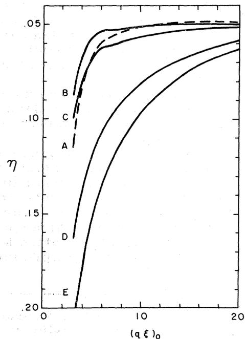
FIG. 3. Exponents  $\eta$  obtained by a least-squares fit for scattering angles from  $(q\xi)_0$  to  $10(q\xi)_0$  with intensities calculated for  $\eta=0.05$  with the Fisher-Aharony equation on the critical isochore (curve A) and with the Tarko-Fisher equation on the critical isochore (curve B), for  $\theta=0.2$  (curve C), for the critical isotherm (curve D), and for the coexistence curve (curve E). The curve for  $\theta=0.4$  lies between curves B and C.
