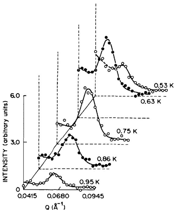
FIG. 2. SANS peak from  $(\text{Er}_{0.8}\text{Ho}_{0.2})\text{Rh}_4\text{B}_4$  at various temperatures.
