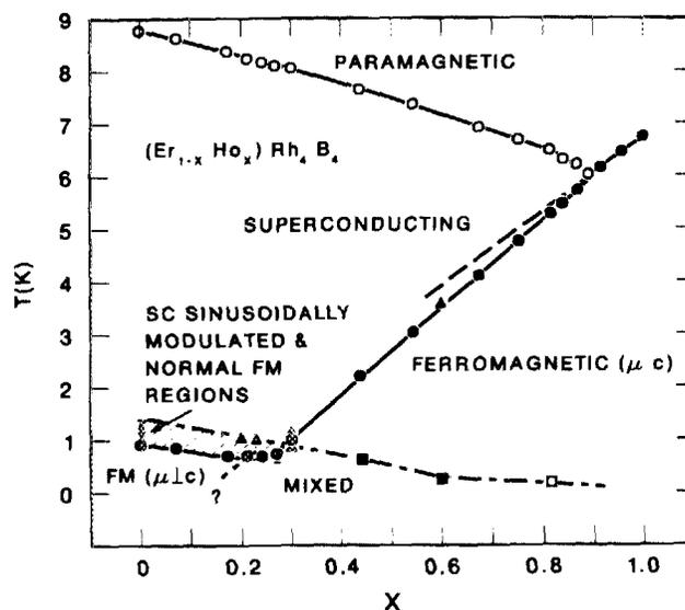
FIG. 1. Low-temperature phase diagram for the  $(\text{Er}_{1-x}\text{Ho}_x)\text{Rh}_4\text{B}_4$  system.<sup>1</sup>
