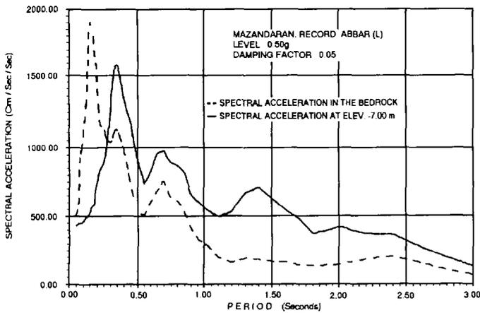
Fig. 5. Spectral acceleration diagram of the region at the level 0.5 g.
