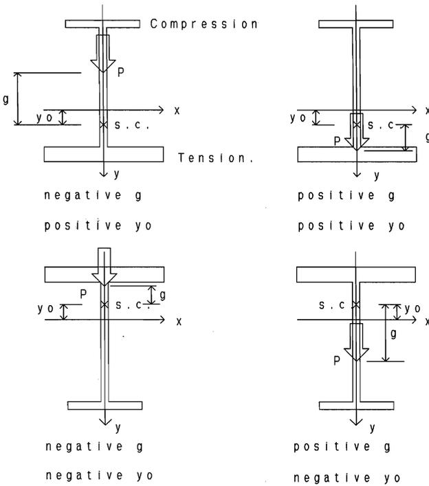
Fig. 2 Orientation of the axes and cross-sectional notation
