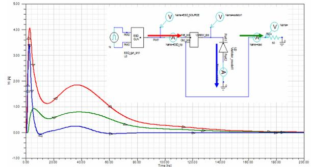
Fig. 7 Simulated ESD current waveform with the varistor
