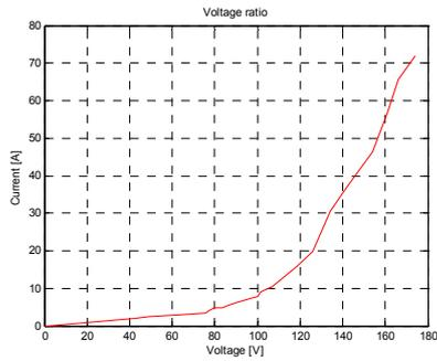
Fig. 4 Voltage vs. current of a varistor
