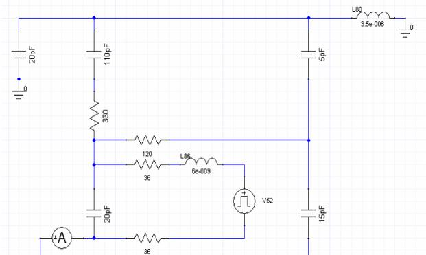
Fig. 1 Equivalent circuit model of the ESD generator
