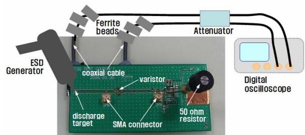
Fig. 3 Test PCB with the varistor mounted
