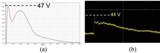
Fig. 9 Voltage waveform comparison: (a) simulated; (b) measured
