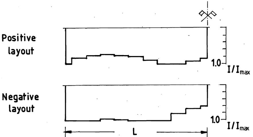
Fig.5 Variation of the moment of inertia
