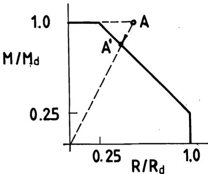
Fig. 3 Moment - support reaction interaction (EC3-Annex A)
