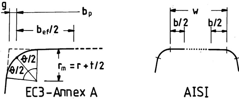
Fig. 1 Definition of the "basic width"
