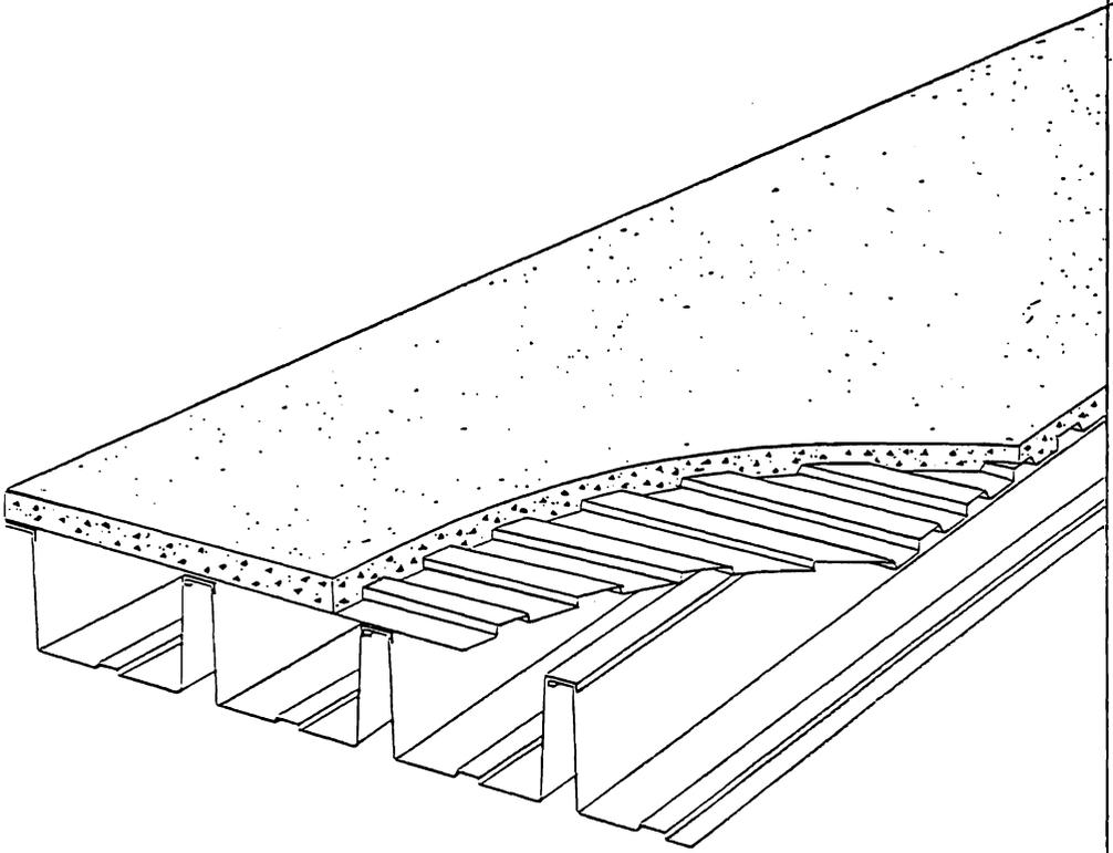
**Figure 1. Long-Span Cold-Formed Deck/Concrete Slab Composite Floor System**
