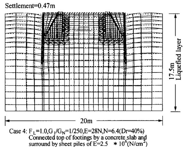
Fig. 14. Deformation of footings and ground in Case 4
