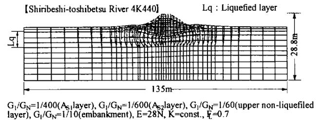
Fig. 5. Deformation of the river levee at Site No.9 of Shiribeshi-toshibetsu River (Yasuda et al., 2000a)
