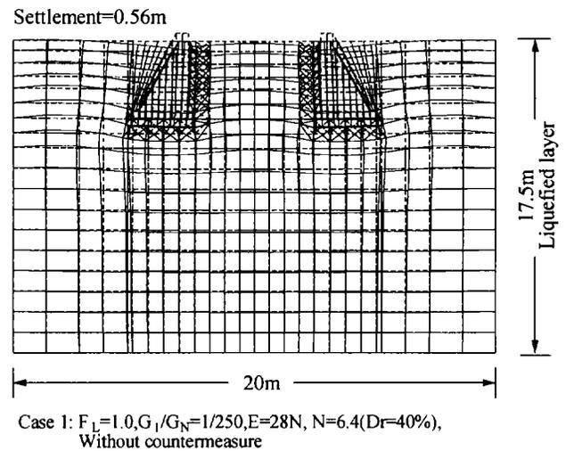
Fig. 13. Deformation of footings and ground in Case 1
