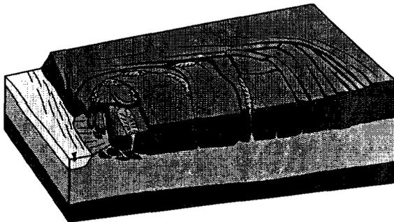
Fig. 1. Schematic depiction of a lateral spread.
