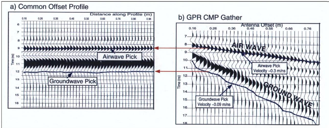
**Figure 3.** (a) Short section of a common-offset GPR profile showing air- and ground-wave events; (b) GPR CMP gather corresponding to common-offset profile, showing how events identified on the CMP gathers can facilitate identification of the same events on co-located common-offset data. Once the events are identified on the GPR common-offset data, they can be easily picked over the entire grid and the traveltime differences used to estimate near-surface volumetric water content.
