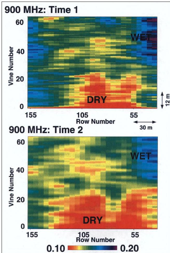
**Figure 5.** Comparison of volumetric water content estimates from 900-MHz common-offset GPR ground-wave data over the entire study area shown in Figure 1 during two different times of the year. These images reveal a persistence of near-surface water content spatial distribution at the site, which we interpret to be controlled by near-surface soil texture.
