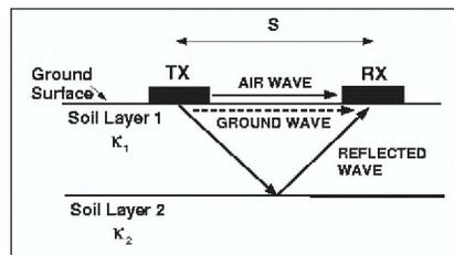
Figure 2. Air, ground, and reflected GPR energy travel paths.  $S$  is the separation distance between the transmitter (Tx) and receiver (Rx), and  $\kappa$  is the dielectric constant of the upper ( $\kappa_1$ ) and lower ( $\kappa_2$ ) geologic layers.
