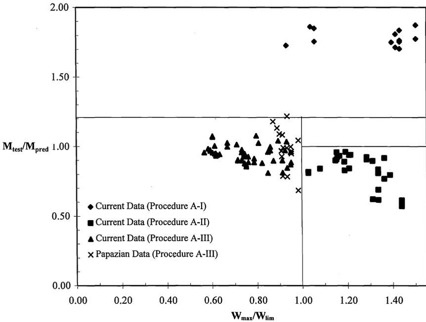
**Figure 2 -  $M_{test}/M_{pred}$  vs.  $W_{max}/W_{lim}$  (AISI 96)**
