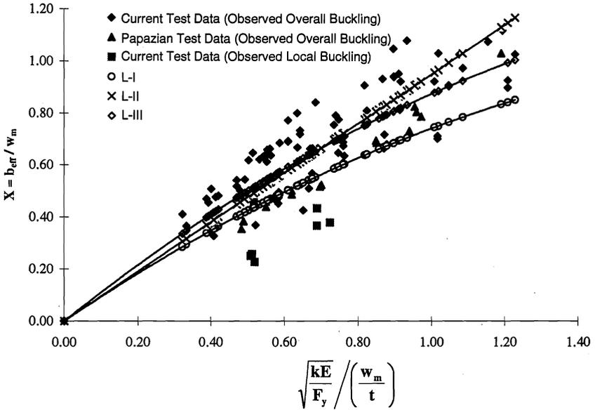
Figure 3 - Compression Flange Width Reduction Factor  $\chi$  vs. Modified Lind Procedures
