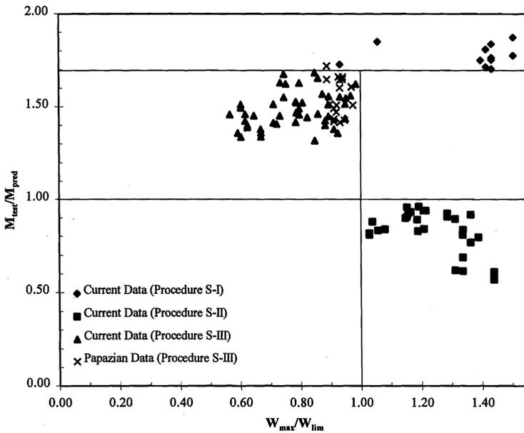
Figure 1 -  $M_{test} / M_{pred}$  vs.  $W_{max} / W_{lim}$  (S136-94)
