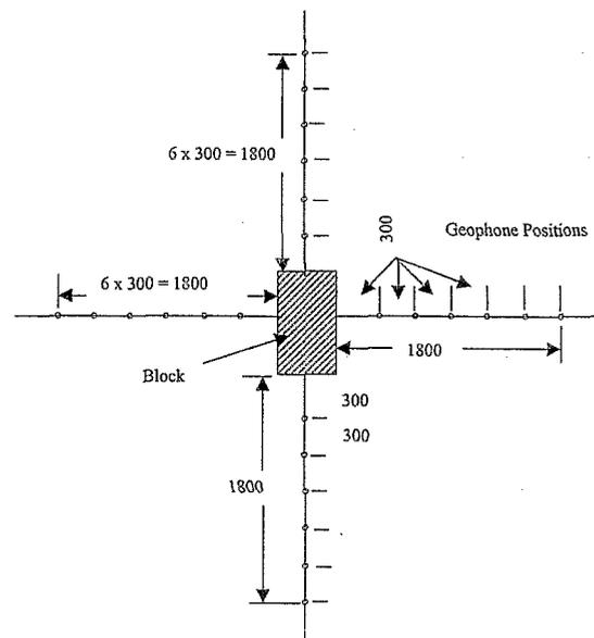
**Fig. 2 Plan showing Locations of Ground vibrations observations**
