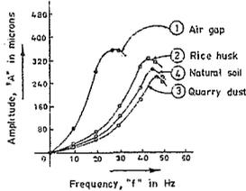
FIG. 6. RESPONSE CURVES OF BACKFILLS AT  $\alpha = 50^\circ$
