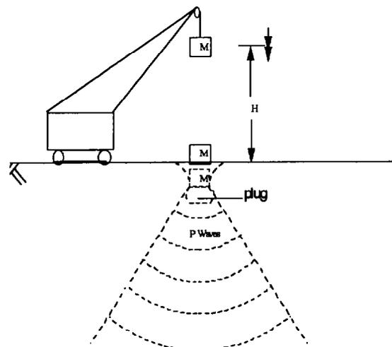
Figure 1 Dynamic compaction
