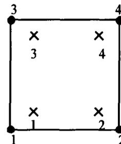
Figure 3 First-order 4-node bilinear axisymmetric quadrilateral finite element
