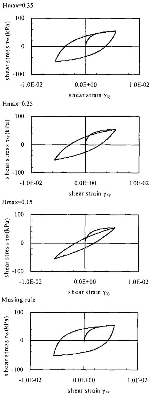
Fig.5 Shear stress – shear strain relationships (computed):
