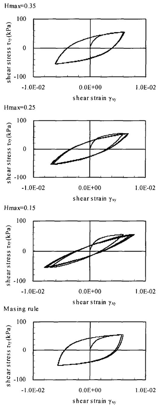
Fig.6 Shear stress – shear strain relationships (computed):
