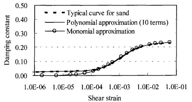
Fig.3a Typical damping characteristics of sand obtained empirically and its approximated curves
