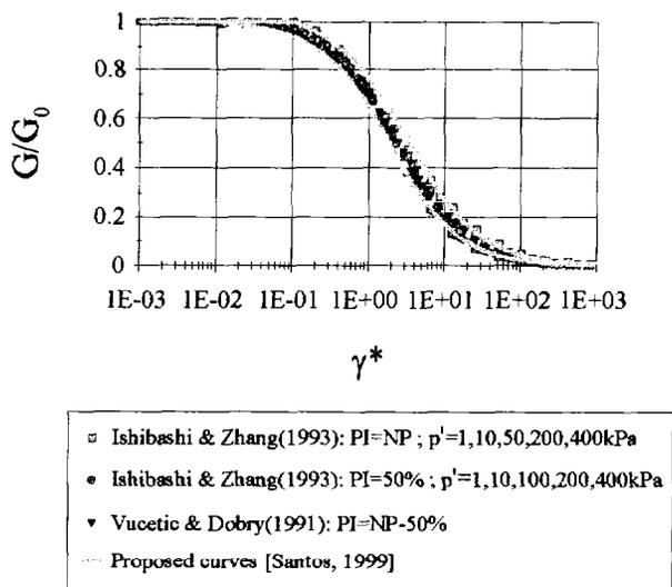
Figure 1 – Stiffness degradation curves in  $\gamma^*$  scale
