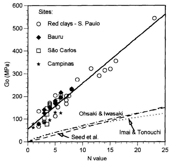
Figure 4. Experimental data for lateritic soils and correlations obtained from temperate zone soils (Barros, 1997<sup>a</sup>)
