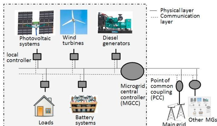
Fig. 1. A microgrid with renewable energy sources
