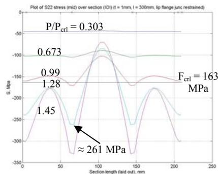
**Figure 12 Longitudinal stress around section (forced local)**
