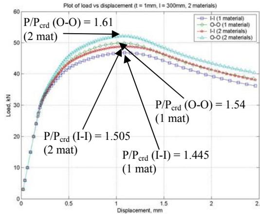
**Figure 14 Load deflection curve for section  $t=1\text{mm}$  (2 materials)**
