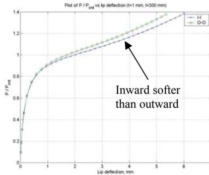
**Figure 11 Plot of  $P/P_{\text{crd}}$  vs lip deflection for section  $t = 1\text{ mm}$**
