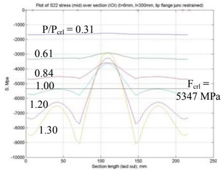
**Figure 8 Longitudinal stress around section (forced local)**
