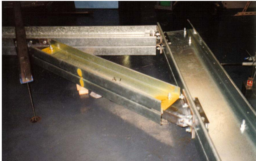
Figure 11 View of stanchion-rafter brace
