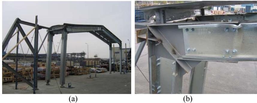
Figure 10. C1 frame: global view (a) and local buckling of the left beam connection (b).
