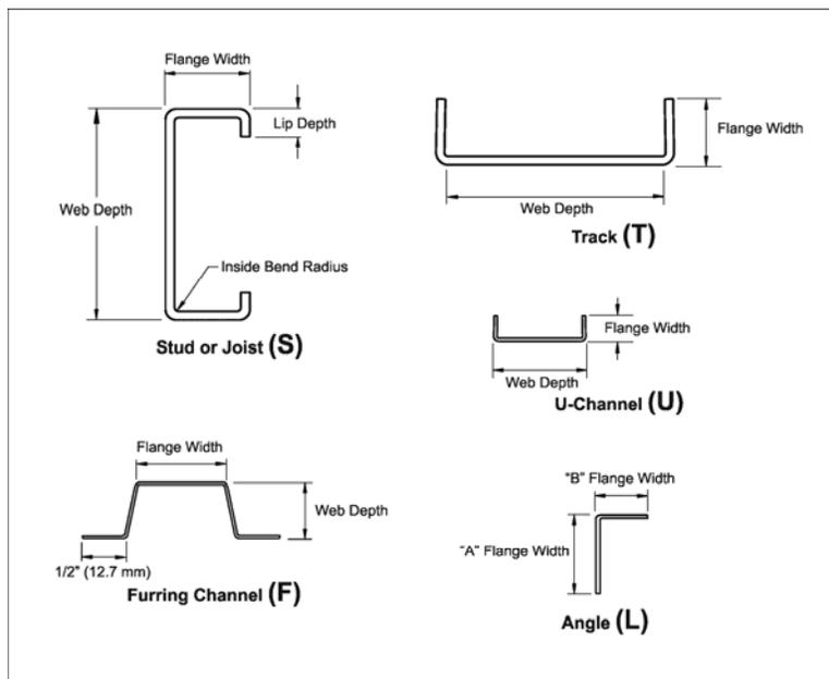
Figure 2: Cold Formed Steel Framing Member Types
