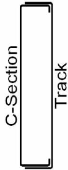
Figure 1: Typical hip and ridge member configuration
