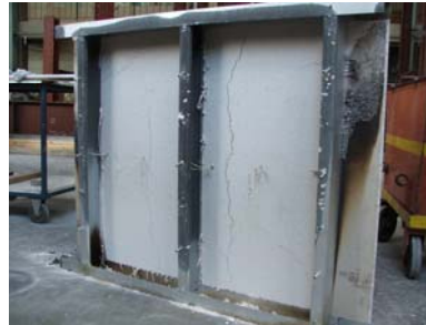
Figure 4: Failure of Test Specimen 1 built without insulation
