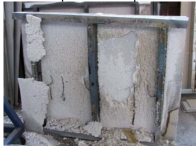
Figure 5: Failure of Test Specimen 2 using glass fibre as cavity insulation
