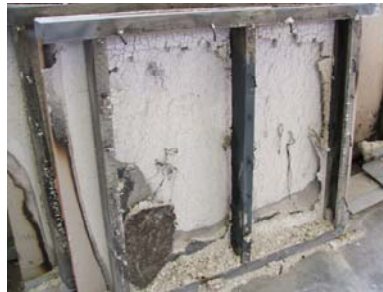
Figure 6: Failure of Test Specimen 3 using glass fibre as external insulation
