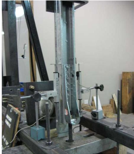
Figure 6 – Raised hold-down Assembly Tension Test Setup – Front
