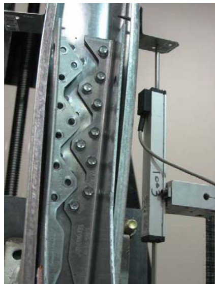
Figure 7 - Hold-down Assembly Tension Test Failure – Screw Shear
