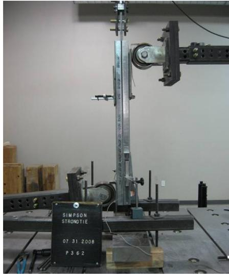
**Figure 5 – Raised hold-down Assembly Tension Test Setup – Side**
