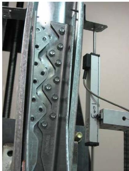
Figure 7 - Hold-down Assembly Tension Test Failure – Screw Shear
