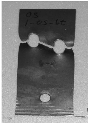
(a) Two-bolt Specimen Failure
