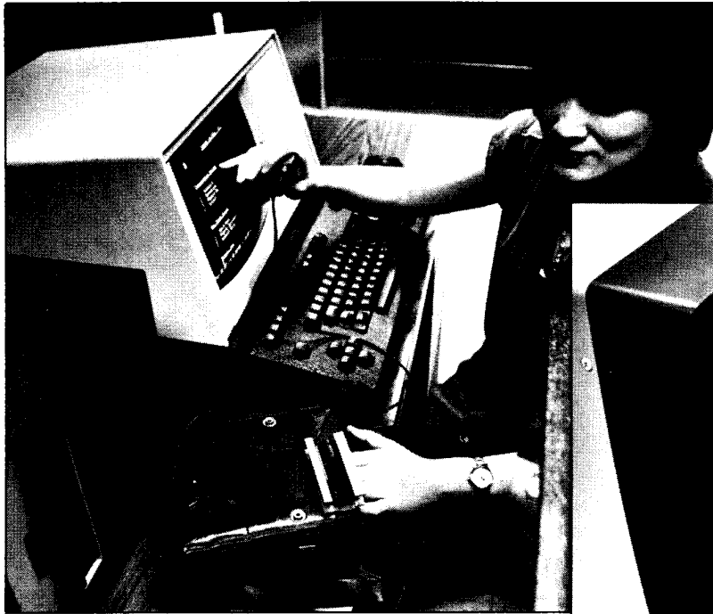
This woman is reading the screen with a product called Optacon (Optical Tactile Converter), conceived by IEEE Life Fellow John G. Linvill. As the lens module moves across the image of a character, it converts the shape of the light onto a tactile array of vibrating rods, which can be scanned by the touch of a finger.
