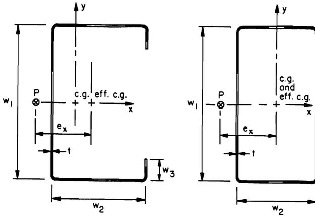
Fig. 1 Section geometry and generalized effective section
