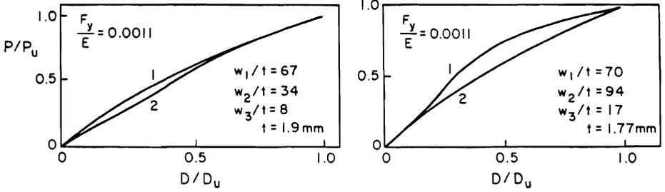
Fig. 4 Evaluation of stub column test results
