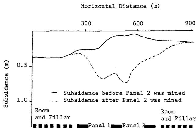
Figure 2. Transverse Profiles of a Case Study Showing the Influence of the Adjoining Room and Pillar Sections
