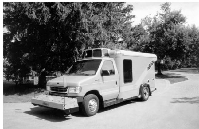
**FIGURE 4** Roof-mounted video for panoramic view.
