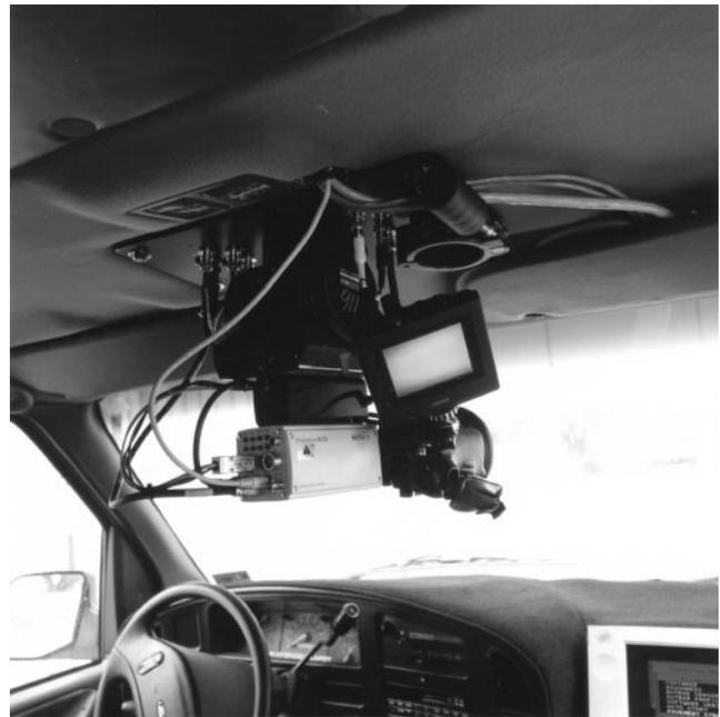
**FIGURE 3** Cab-mounted video camera in data collection vehicle.
