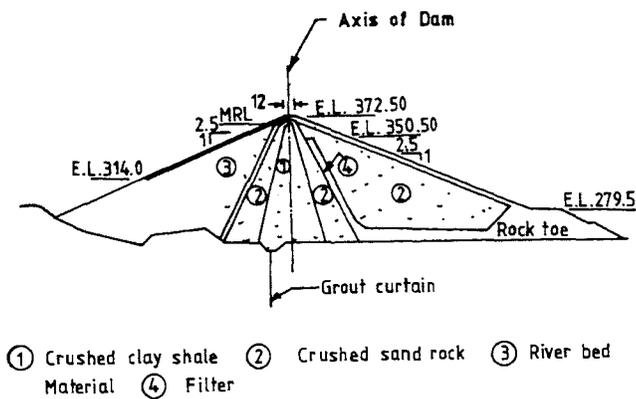
Fig. 3. Cross-section of Ramganga Dam
