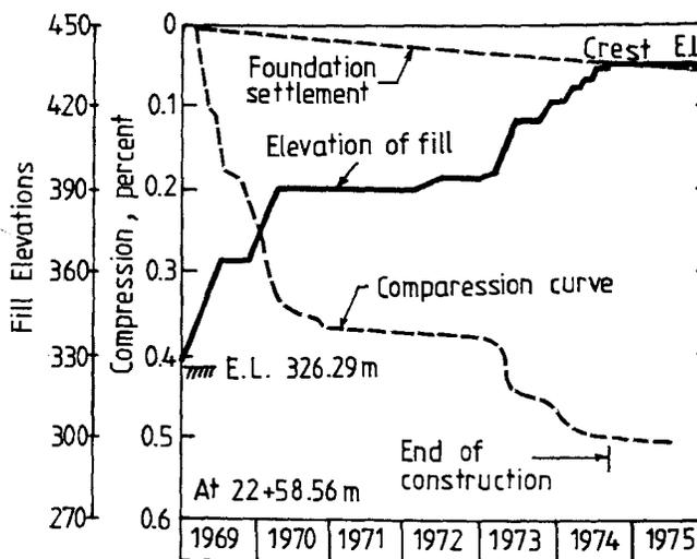
Fig.2. Typical Foundation and Embankment Response of Beas Dam
