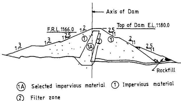
Fig.7. Cross-section of Tawa Dam
