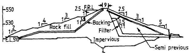
Fig. 5. Cross-Section of Linganamakki Dam
