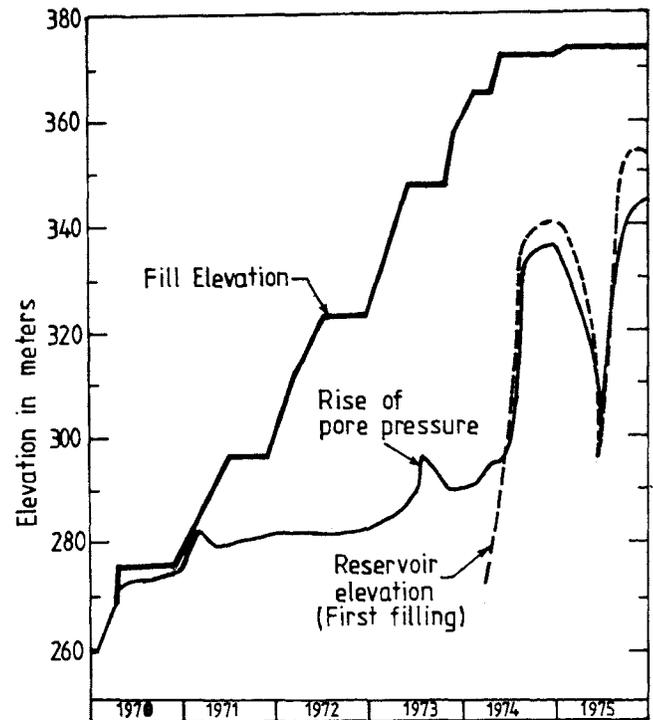
Fig. 4. Pore Pressure Response in Shell Zone of Ramganga Dam due to Embankment Construction and Reservoir Filling
