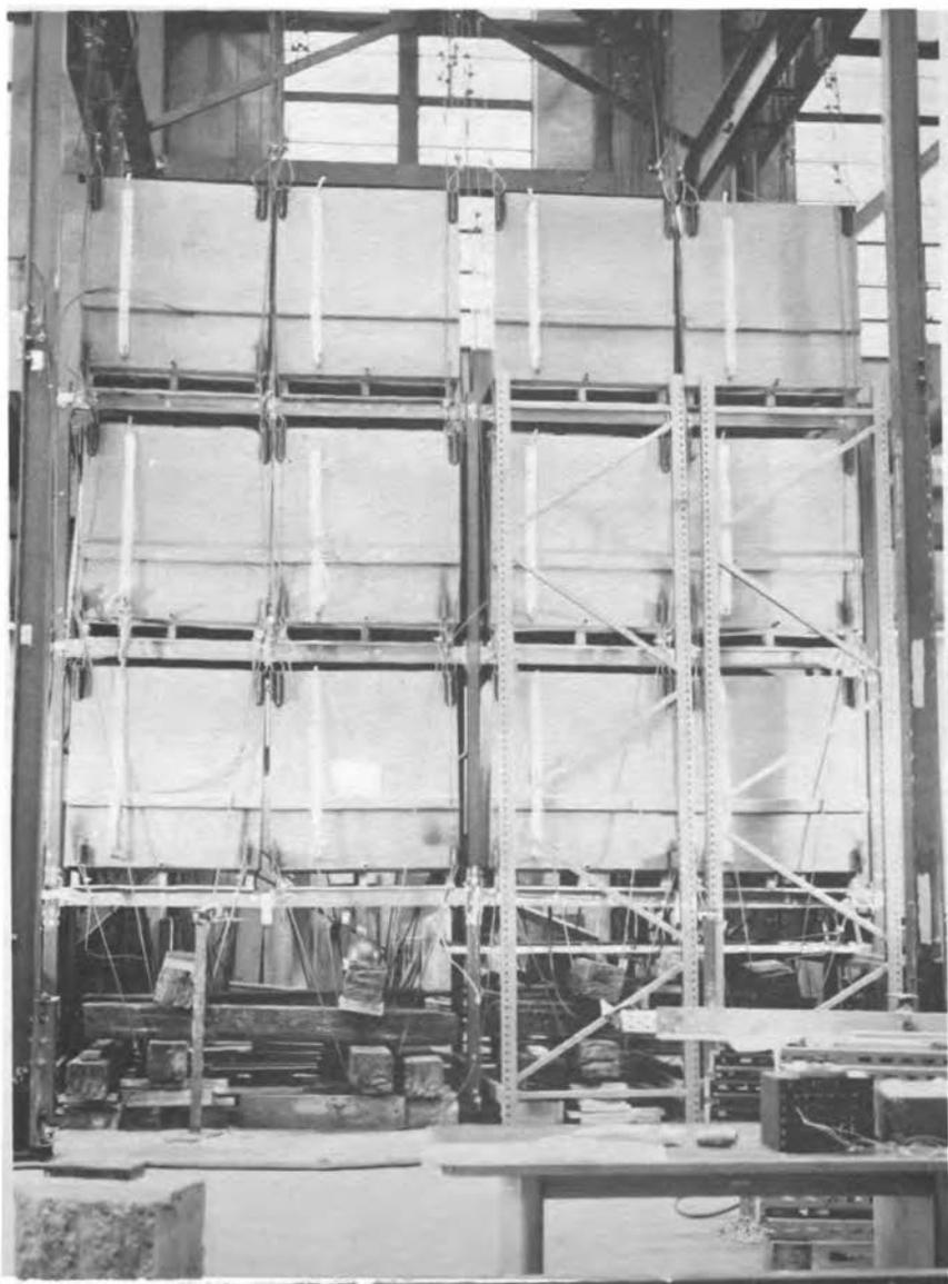
Fig. 3 Overall View of Tested Type B Rack
