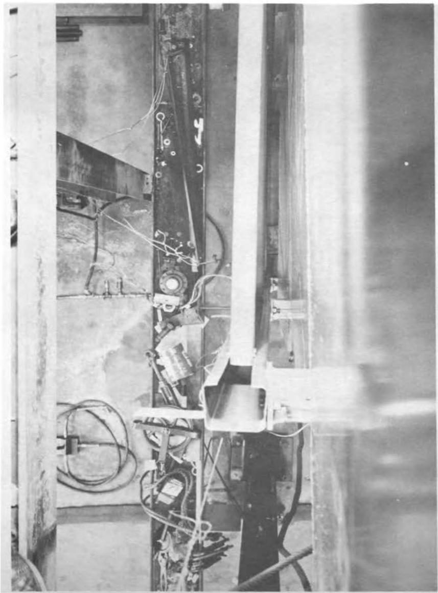
Fig. 5 Top View of a Post of Type B Rack
