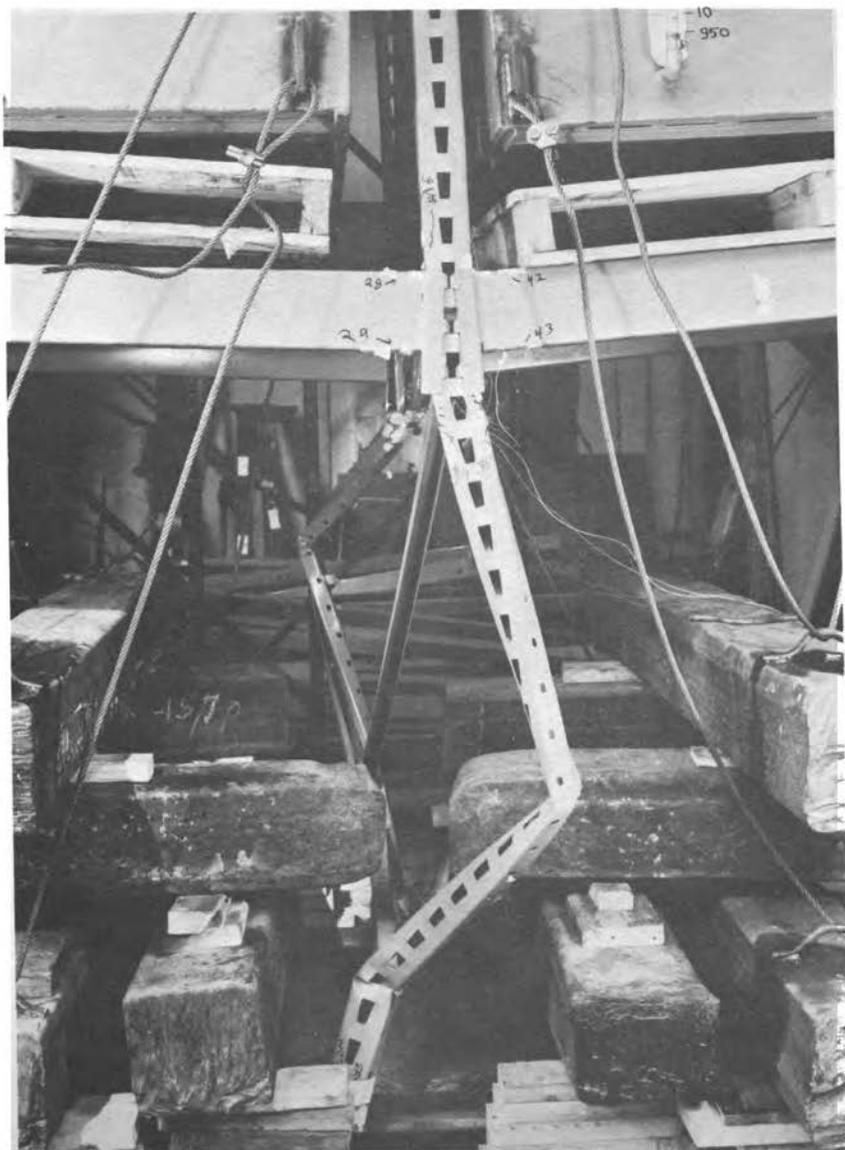
Fig. 7 Close-up View of the Center Upright of Tested Type B Rack - Vertical Loading Only
