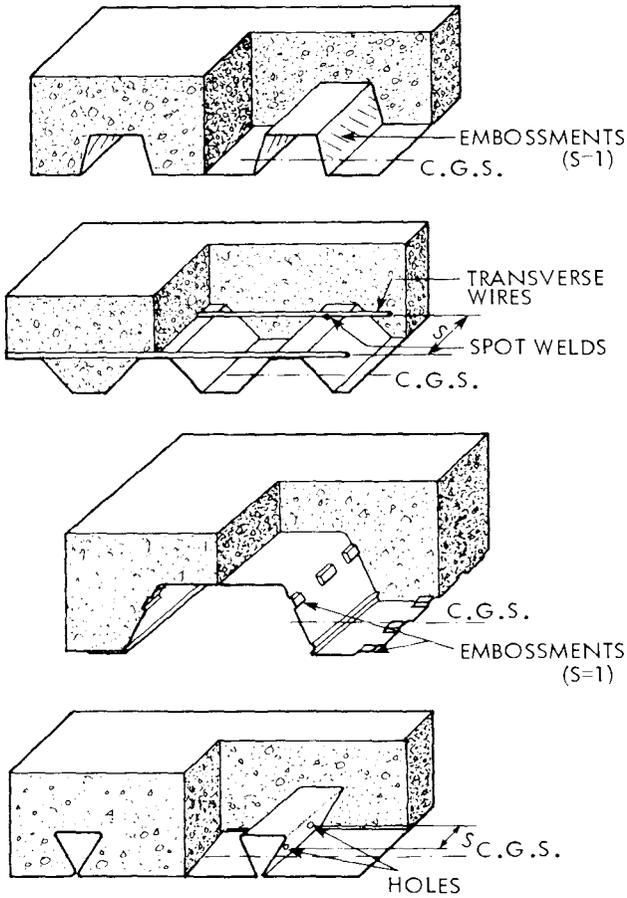
Fig. 2. Examples of composite steel-deck floor slab systems.
