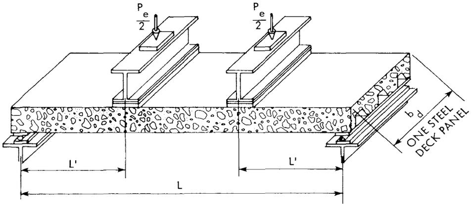
Fig. 5. Typical arrangement for testing one-way slab elements.
