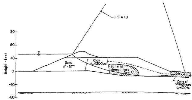
Fig. 6 Probable Condition of Upper San Fernando Dam just after 1971 San Fernando Earthquake
