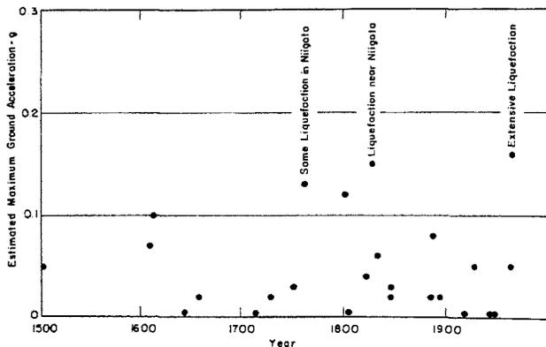
Fig. 5 Estimated Peak Ground Accelerations Developed by Earthquakes in Niigata, Japan
