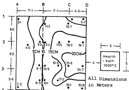
Fig. 2 Contours of Heave of Ground Floor (February, 1977)
