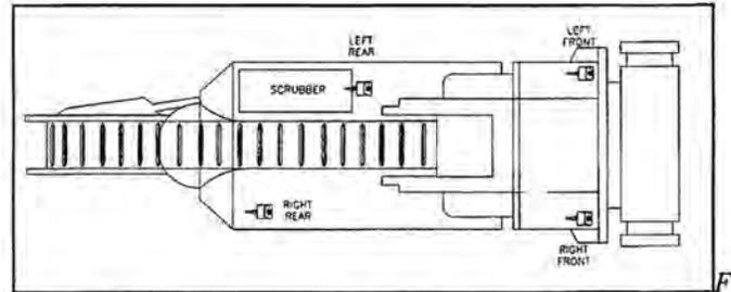
Figure 2. Typical monitoring positions on a CM.
